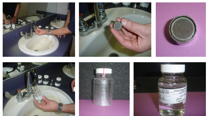
Figure 2: Water sampling for microbiological testing. Remove the aerator from the faucet before collecting the sample. Collect a water sample in a sterile container and cap immediately. (Bottom Center): Sterile bottle with tamper-proof seal. Contains white powder - DO NOT REMOVE. (Photos: authors)
